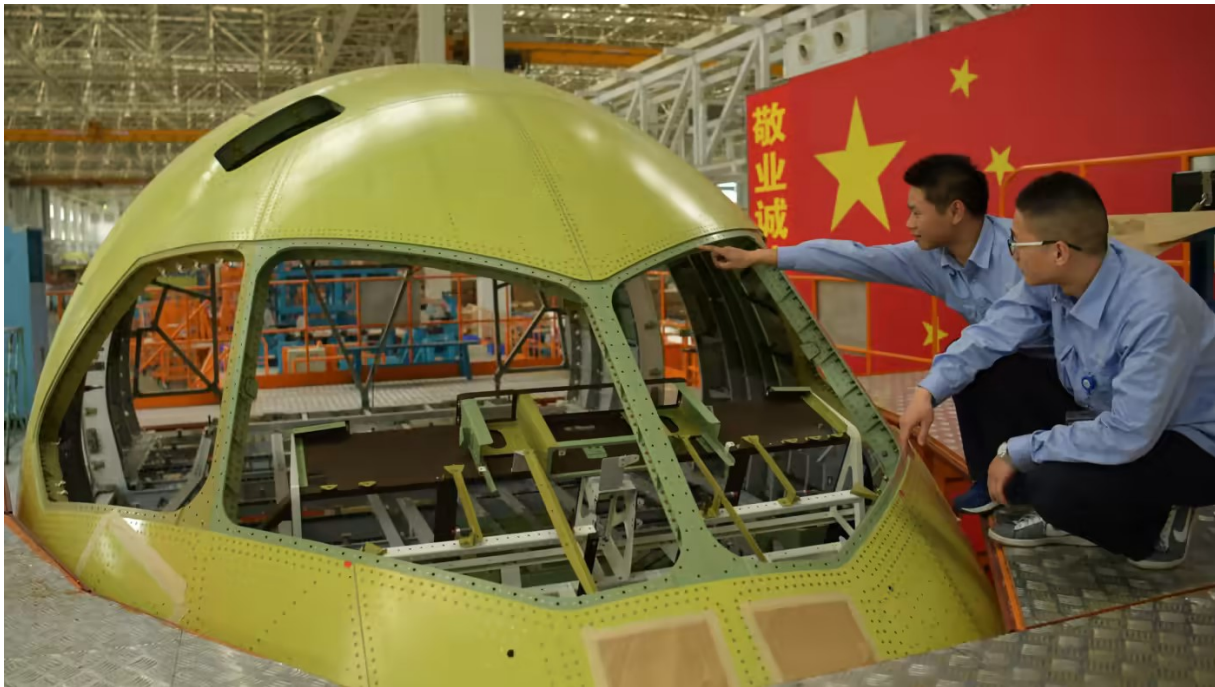
Workers stand outside the cockpit section of China's third C919 passenger jet during construction © AFP/Getty Images
