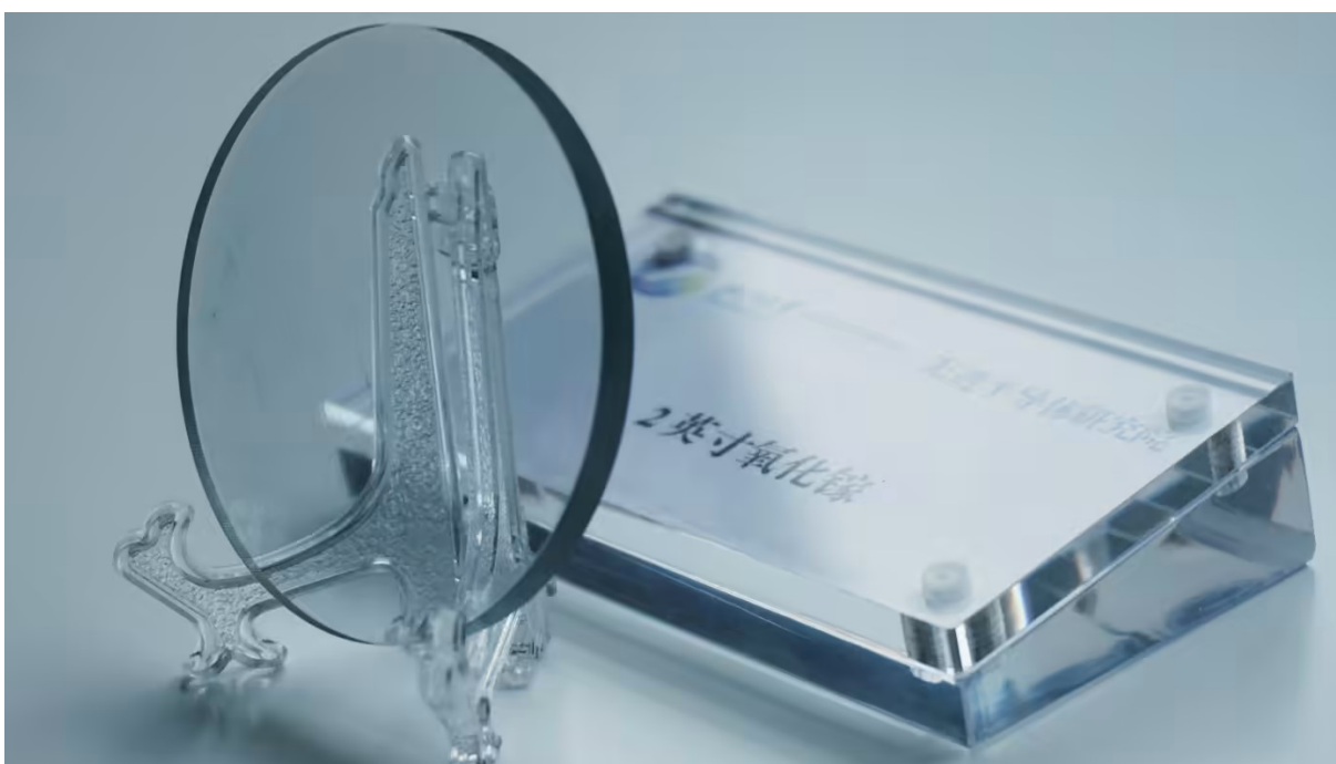
A gallium oxide wafer at Zhejiang University in China. The US and China are locked in a battle for technology supremacy © Cynthia Lee/Alamy
