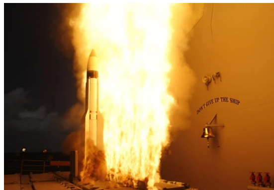
The advanced SM-3 missile has been designed to intercept ballistic missiles either in midcourse or terminal phase.
