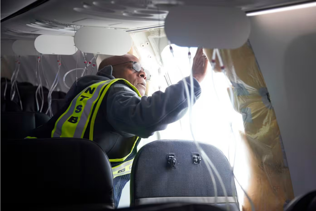
An investigator examines a section of the Alaska Airlines aircraft that had experienced a mid-air blowout of a door plug on the fuselage, leading to the temporary grounding of Boeing’s Max 9s © NTSB/AP
