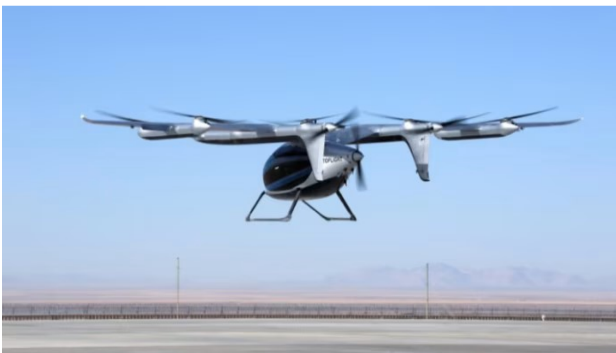
AutoFlight's Prosperity flying taxi can carry up to five people. The vehicles take off vertically like a helicopter then transition into fixed-wing mode to travel at high speed © AutoFlight
