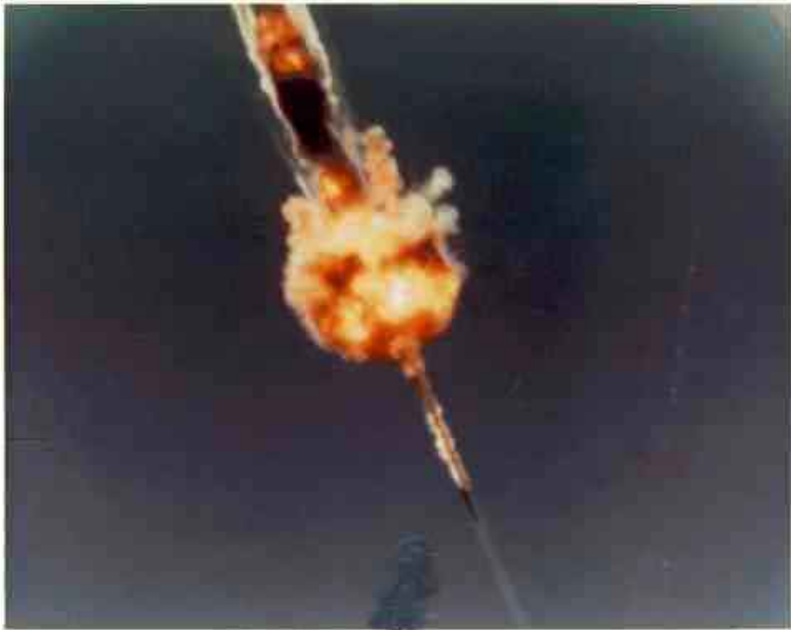
Figure B-I: A Patriot intercept attempt on a Lance missile at the White Sands Missile Range. The Patriot has damaged the control surfaces of the Lance (which will later cause it to tumble), but otherwise the Lance is intact. A measurement of the length to diameter ratio of the Lance (a Lance is about 6.14 meters long and 0.56 meters in diameter) indicates that the Lance is not significantly foreshortened by viewing angle effects (alternatively, the fireball diameter can just be measured with respect to the Lance diameter). The fireball diameter is four to five times the Lance length, or about 25-30 meters.
