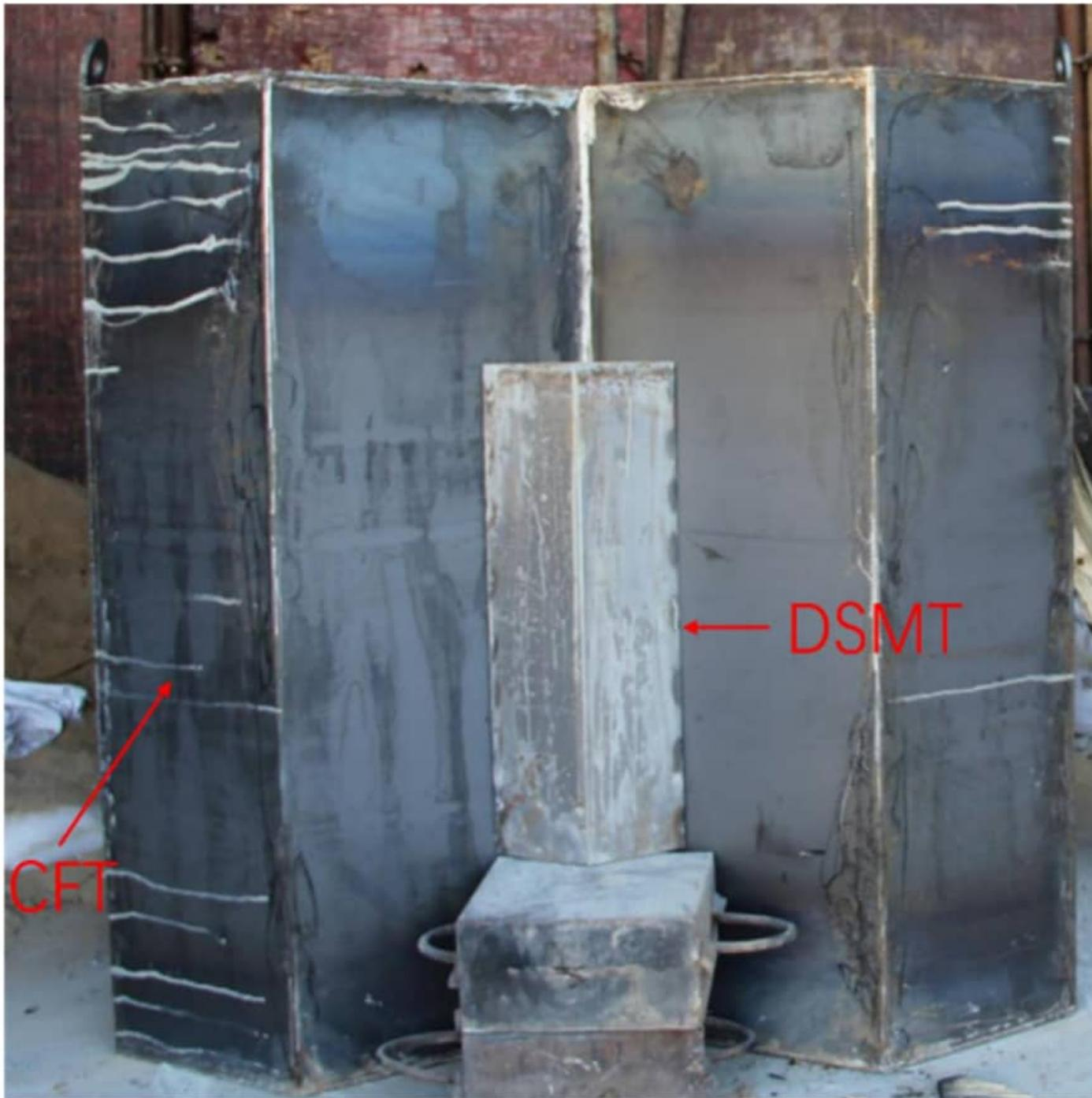
Figure 5. Photograph of the composite target plate with diamond-shaped moving target.
