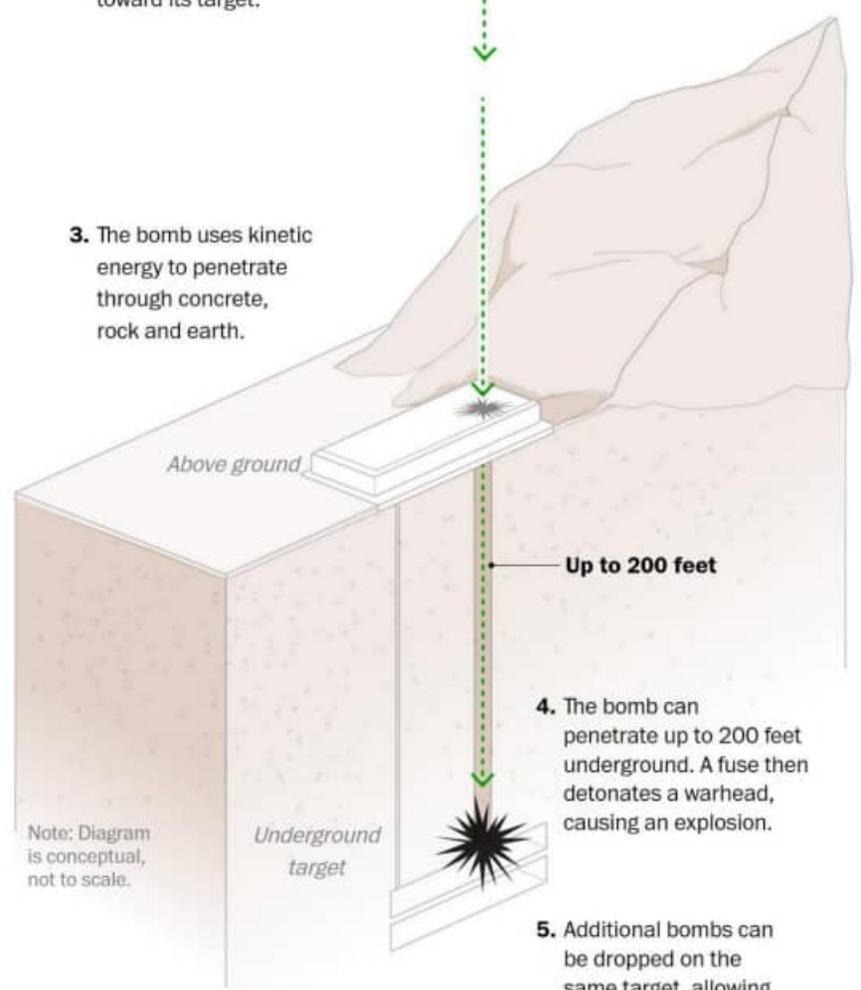
4. The bomb can penetrate up to 200 feet underground. A fuse then detonates a warhead, causing an explosion.
